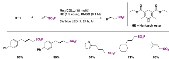
Scheme 31 Selected examples for the photocatalyzed syntheses of fluorosulfonylated alkyl compounds from alkyl iodides.
