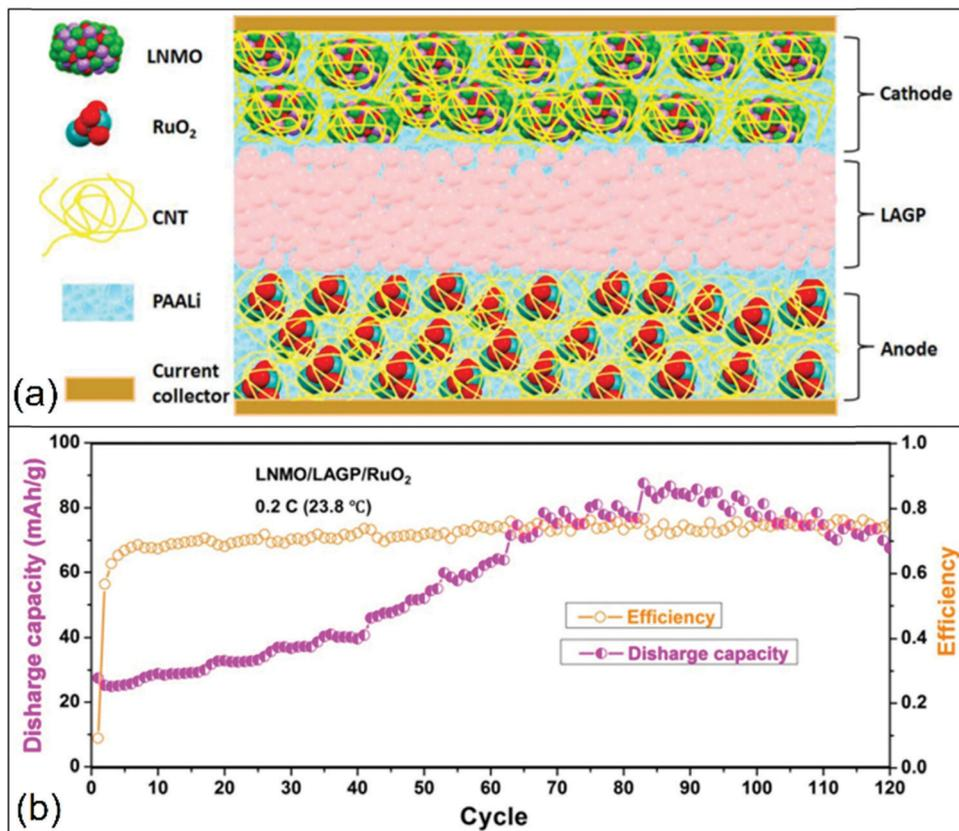
Fig. 19 (a) Schematic illustration of the full lithium-ion solid-state battery using LNMO/CNT/PAALi as the cathode, LAGP as the solid electrolyte, and RuO<sub>2</sub>/CNT/PAALi as the anode, where both sides were sputtered with gold as current collectors. (b) Discharge capacity and efficiency of LNMO/LAGP/RuO<sub>2</sub> at room temperature at 0.2C using PAALi as a binder.<sup>408</sup> Reproduced with permission from The Royal Society of Chemistry, UK.<sup>408</sup>
