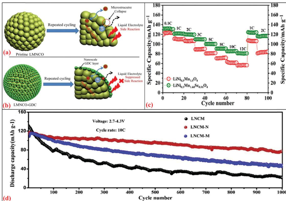
Fig. 8 Schematic illustrations of (a) pristine LMNCO interfacial side reactions with liquid electrolyte after repeated cycling<sup>244</sup> and (b) GDC coating layer acts as a protection layer to suppress the unwanted interfacial side reactions after repeated cycling.<sup>245</sup> (c) Rate capability for LNMO and LNMSO cathode for 0.1–12C. (d) Cycling performances for LNCM, LNCM-N, LNCM-M at C-rate of 10C.<sup>246</sup> Reproduced with permissions from Elsevier.<sup>244–246</sup>
