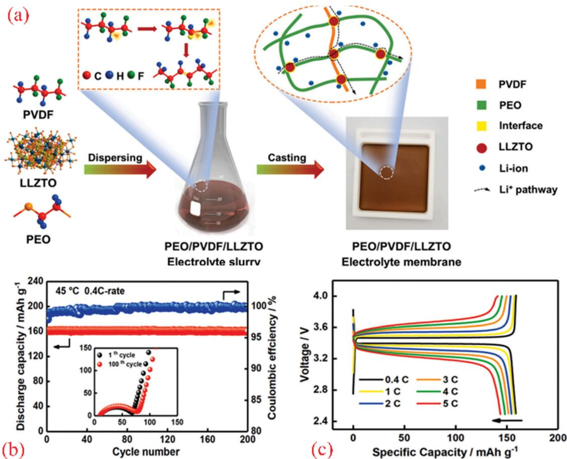
Fig. 21 (a) Fabrication process of the PLFF (PEO/PVDF/LLZTO/LiTFSI) solid composite electrolyte. (b) Cycling performances at 0.4C and 45 °C and the impedance of LiFePO<sub>4</sub>/Li cell cycling with PLFY. (c) Different rates of galvanostatic charge–discharge profiles of LiFePO<sub>4</sub>/PLFY/Li cells under 45 °C.<sup>358</sup> Reproduced with permission from Elsevier.<sup>358</sup>
