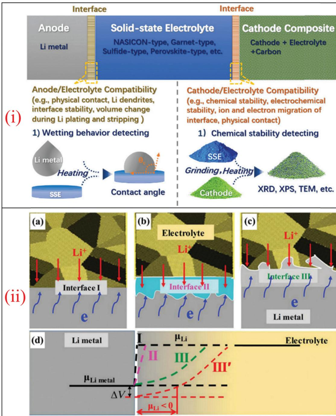
**Fig. 16** (i) Summary of compatibility problems associated with interfaces in SSBs (Fig. 1 from ref. 322). (ii) Formation of different types of Li/SSE interphases. (a) Intrinsically stable interface between the Li metal and the SSE. (b) Metastable solid-electrolyte interphase between the Li metal and the SSE. (c) Reactive mixed-conducting interphase between the Li metal and the SSE. (d) Corresponding Li potentials between the Li metal and different SSEs.<sup>322</sup>
