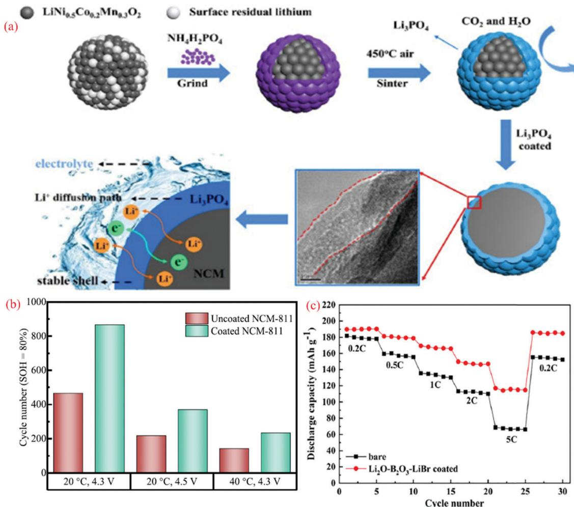
Fig. 7 (a) Schematic diagram of the experimental process.<sup>219</sup> (b) Achieved cycle numbers for different cycling conditions at an SOH of 80%. The calculation of the SOH is based on the capacity of the fifth cycle and (c) rate performance for uncoated NCM 523 and  $\text{Li}_2\text{O}-\text{B}_2\text{O}_3-\text{LiBr}$ -coated NCM523. Reproduced with permission from Elsevier.<sup>219</sup>
