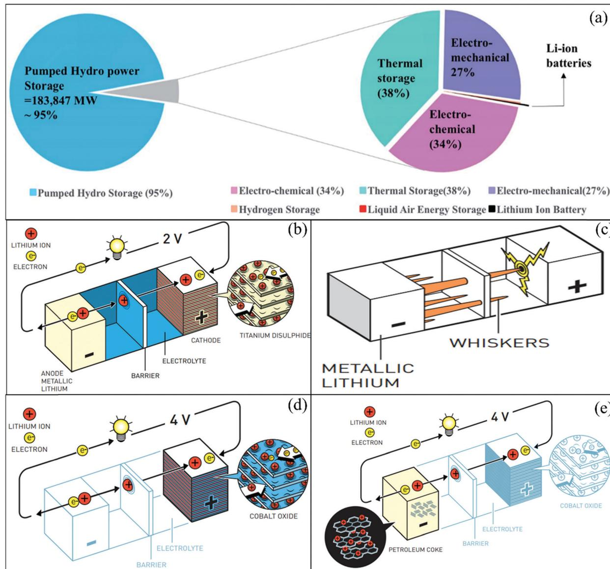
Fig. 2 (a) Contribution of worldwide energy storage projects to grid applications.<sup>30</sup> (b) Lithium-based battery using  $\text{Li}_x\text{TiS}_2$  as the cathode. (c) Formation of lithium whiskers/dendrites potentially leading to short-circuiting. (d) Lithium-based battery using  $\text{Li}_x\text{CoO}_2$  as the cathode. (e) Ion transfer cell lithium-ion battery configuration. (©Johan Jarnestad/Royal Swedish Academy of Sciences<sup>33</sup>).
