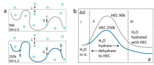
Fig. 6 Illustration of the possible mechanism for hydration and dehydration in electrolytes with different HECs. (a) The two steps of water absorption into the electrolytes containing HEC 90k (top) and HEC 250k (bottom). (b) The Gibbs energy of hydration/dehydration in IL with HEC 90k and 250k.
