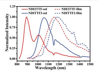
Fig. 2 Normalized emission spectra of the CHCl $_3$  solutions (solid lines) and thin films (dashed lines) of **NDITTF2** and **NDI2TTF**. The concentration for each molecule was 10  $\mu$ M and the excitation wavelength was 808 nm.
