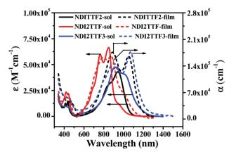
Fig. 1 Absorption spectra of chloroform solutions (solid lines) and thin films (dashed lines) of NDITTF2, NDI2TTF and NDI2TTF3. The concentration for each molecule was 10 µM.
