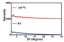
Fig. 5 XRD pattern of the as-cast thin-film of NDITTF2 and that after annealing at 160 °C for 15 min.
