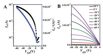
Fig. 4 The transfer and output characteristics of the FET device based on NDITTF2 after being annealed at 160 °C for 15 min. The transistor channel width and channel length were 1440 μm and 40 μm, respectively
