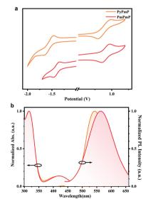
Fig. 2 (a) Cyclic voltammetry curves of PyPmP and PmPmP measured in DMF, and (b) their normalized absorption and emission spectra in dilute toluene at ambient temperature Molecular structures of PyPmP and PmPmP and their simulated HOMO/LUMO energy levels and spatial distributions. The isovalue is 0.02.
