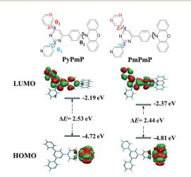
Fig. 1 Molecular structures of PyPmP and PmPmP and their simulated HOMO/LUMO energy levels and spatial distributions. The isovalue is 0.02.
