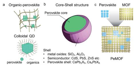
Fig. 2 Perovskite nanocrystal developed in the field. Schematic illustration of (a) examples of organic-perovskite nanocrystal structures, (b) core—shell structure to confine the perovskite nanocrystals and (c) perovskite/MOF structure by confining the perovskite nanocrystal in a MOF matrix.
