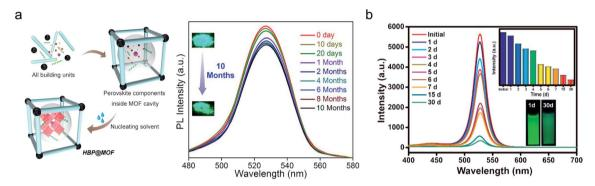
Fig. 5 Moisture stability of PeMOF. (a) PeMOF structures developed by Mollick et al., where the emission from the perovskite remains strong over 10 months of air exposure, Reprinted with permission from ref. 103, Copyright 2019 American Chemical Society, (b) Photoluminescence spectra of the PeMOF developed by Zhang et al., which exhibits robust emission when immersed in water for 30 days. Reprinted with permission from ref. 102. Copyright 2018 American Chemical Society.
