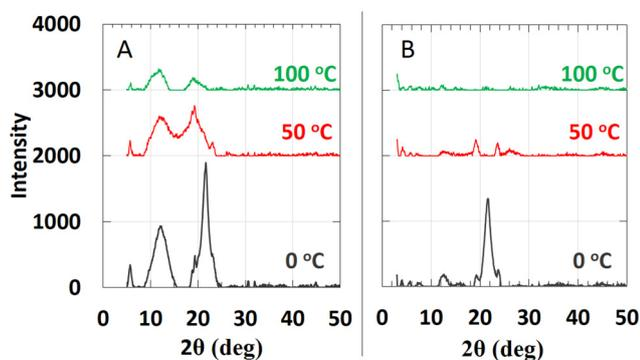
Fig. 5 Variable temperature PXRD diffractograms of 2-18: (A) starting at 0 °C, 2-18 was heated from 0 to 100 °C; (B) after 5 days at room temperature, 2-18 was again heated from 0 °C to 100 °C.
