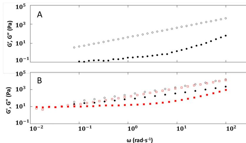
Fig. 6 Moduli versus angular frequency sweeps ( $\omega$ ) of imidazolinium ionomers with hexyldithiocarbamate and octadecyldithiocarbamate anions: (A) **2–6** ( $\bullet = G'$ ,  $\circ = G''$ ), at 25 °C and 1% strain; (B) **2–18** ( $\bullet = G'$ ,  $\circ = G''$ ) at 40 °C and 0.5% strain and **2–18** ( $\blacksquare = G'$ ,  $\square = G''$ ) at 50 °C and 0.5% strain.
