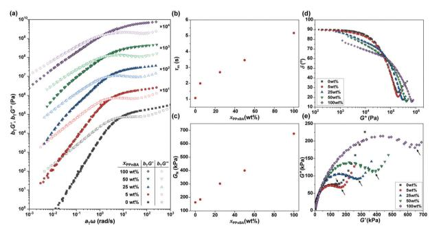
Fig. 3 (a) Master curves of storage (G') and loss (G") moduli for PnBA/PPnBA blended elastomers at the reference temperature of 20 °C. The data are vertically shifted for clarity using the multiplication factors shown in the plot. (b) Relaxation time of the melt ( $\tau_m$ ) and (c) plateau modulus ( $G_N$ ) for the PnBA/PPnBA elastomer blend as a function of PPnBA fraction,  $x_{PPnBA}$ . (d) van Gurp-Palmen plots and (e) Cole-Cole plots of the PnBA/PPnBA elastomer
