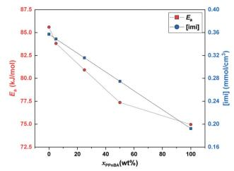
Fig. 4 Activation energy of flow  $(E_a)$  and mole density of imidazole groups ([imi]) as a function of PPnBA fraction,  $x_{PPnBA}$
