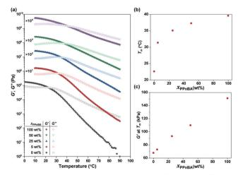
Fig. 2 (a) Temperature-dependence of storage (G') and loss (G'') moduli of PnBA/PPnBA blended elastomers with  $\gamma = 1.0\%$  and  $\omega = 10$  rad s<sup>-1</sup>. The data are vertically shifted for clarity using the multiplication factors shown in the plot. (b) Melting temperature ( $T_{\rm m}$ ) and (c) G' at  $T_{\rm m}$  of the PnBA/ PPnBA elastomer blend as a function of PPnBA fraction ( $x_{PPnBA}$ ).
