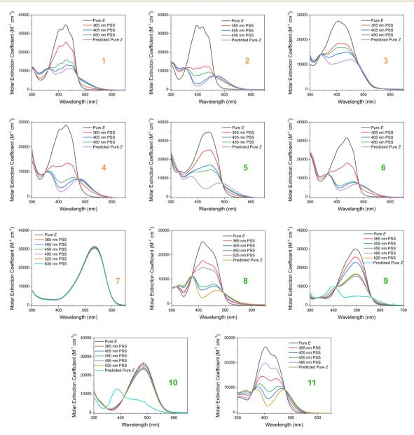
Fig. 5 The experimental UV-vis absorption spectrum of switches 1–11 measured at 25  $\mu$ M in DMSO and shown as the molar extinction coefficient (M<sup>-1</sup> cm<sup>-1</sup>). Different irradiation wavelengths were employed in order to predict the "pure" Z spectra using the procedure detailed by Fischer.<sup>81</sup> The chemical structures of these switches are shown in Fig. 4 above.
