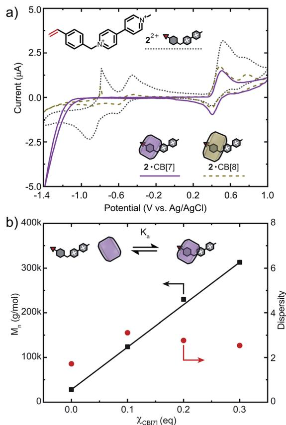
Fig. 5 (a) Cyclic voltammogram of viologen-containing monomer  $2^{2+}$  and its complexation with CB[*n*] ( $n = 7, 8$ ) at a concentration of 1 mM using a scan rate of  $10 \text{ mV s}^{-1}$  in  $0.1 \text{ mM NaCl}$  solution. (b) Molar mass and dispersity of  $2^{2+}$ -containing copolymers *vs.* equivalents of CB[7].  $\text{Cl}^-$  counter-ions are omitted for clarity.
