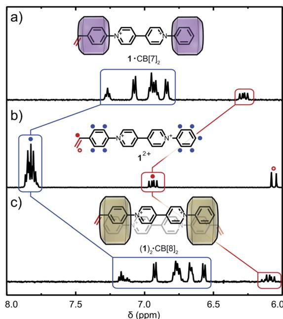
Fig. 2 Supramolecular complexation of  $1^{2+}$  and CB[n]. <sup>1</sup>H NMR spectra of  $1^{2+}$  at (a)  $\chi_{\text{CB}[7]} = 2$ , (b)  $\chi_{\text{CB}[n]} = 0$  and (c)  $\chi_{\text{CB}[8]} = 1$  in D<sub>2</sub>O. Cl<sup>-</sup> counter-ions are omitted for clarity.
