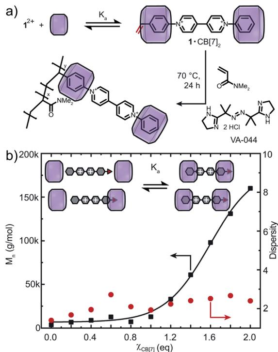
Fig. 3 (a) *In situ* copolymerisation of DMAAm with  $1^{2+}$  and CB[7]. (b) Molar mass and dispersity vs. amount of CB[7] in the system. Fitted curve is drawn to guide the eye.  $\text{Cl}^-$  counter-ions are omitted for clarity.
