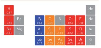
Fig. 7 Initial responses of the electron affinity in a magnetic field as a periodic table representation showing both the numerical values and categorising them with a color code in which blue indicates a positive derivative, red a negative derivative, yellow a derivative that is zero or close to zero and grey those cases where electron affinity was negative and its derivative not computed (see text).
