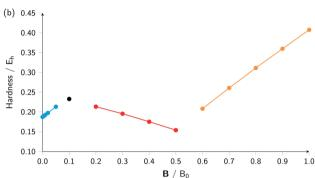
Fig. 2 Electronegativity (a) and hardness (b) *versus* field strength for carbon (all values in a.u.). Different segments correspond to the color codes in Table 2.
