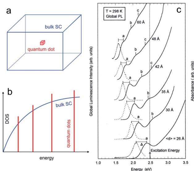
Fig. 2 (a) Scheme showing a 3D bulk SC (blue) and a "OD" quantum dot (red). (b) Density of states (DOS) functions for a bulk SC (blue) and a quantum dot (red). (c) Absorption (solid line) and global PL (dotted line) spectra for InP quantum dots with different mean diameters. The photoexcitation was done at 2.48 eV. Reproduced from ref. 74 with permission from the American Chemical Society, Copyright 1997.
