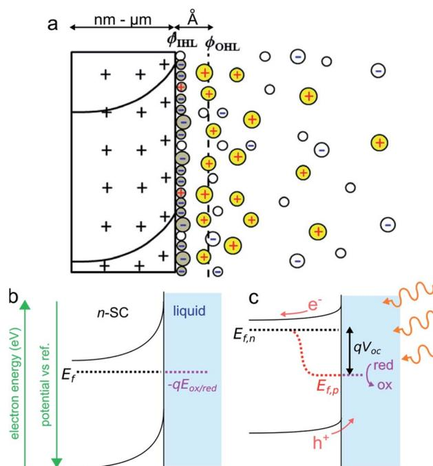
Fig. 3 (a) Scheme of the space charge layer in an n-SC (left) and the Helmholtz layer at the SC/liquid interface (right), adapted with permission from ref. 92  $\phi_{\text{IHL}}$  and  $\phi_{\text{OHL}}$  are the inner and the outer Helmholtz planes. (b) Scheme showing a depleted n-SC in equilibrium with an electrolyte containing the ox/red redox couple in the dark. (c) Scheme showing the effect of illumination ( $h\nu > E_g$ ) on this junction.
