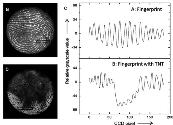
Fig. 5 (a and b) Picture obtained by an ECL-based image-contrast technique showing (a) the image of a latent fingerprint on porous Si, (b) the latent fingerprint impressed with the same fingertip pretreated with TNT. (c) Cross-sectional relative grey scale value over 15 parallel ridges within the area indicated by the black rectangles in (a) and (b). Reproduced from ref. 143 with permission from Wiley-VCH, Copyright 2014.
