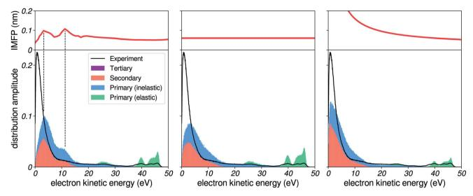
Fig. 6 Influence of the IMFP. Comparison of simulated spectra to experimental results, for a photon energy corresponding to harmonic 37 of ≈800 nm (≈57.6 eV), for several IMFP. Left: extended amorphous ice IMFP. Middle: constant 3 nm IMFP. Right: increasing IMFP at low energies.
