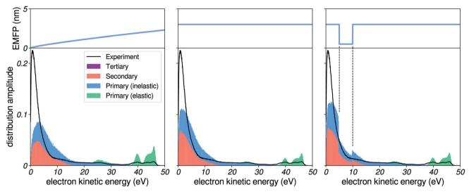
Fig. 5 Influence of the EMFP. Comparison of simulated spectra to experimental results, for a photon energy corresponding to harmonic 37 of ≈800 nm (≈57.6 eV), for several choices of EMFP. Left: EMFP extrapolated from reported results (Fig. 3a). Middle: constant 3 nm EMFP. Right: constant EMFP with a local square-shaped minimum
