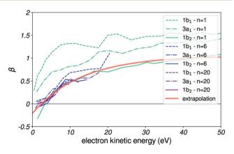
Fig. 12  $\beta$  parameter for photoemission. Experimental  $\beta$  anisotropy coefficient as a function of emitted electron kinetic energy, for n = 1, 6and 20 water clusters and for the three valence orbitals of water. Results reproduced from ref. 49. The red line is the analytical extrapolation used in our simulation.
