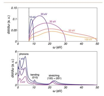
Fig. 4 Singly-differential cross sections for inelastic scattering. Top: SDCS for electronically inelastic events, for incident kinetic energies E=10,20,30,50 and 100 eV. The black vertical line marks the excitation threshold for liquid water. Bottom: SDCS for vibrationally inelastic events, for E=1,2 and 5 eV.
