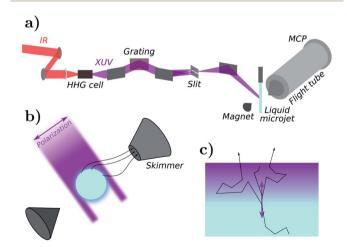
Fig. 1 Photoelectron spectroscopy experiment. (a) Scheme of the experimental setup. (b) Experimental microjet geometry. (c) Semi-infinite flat-surface geometry used in simulations.
