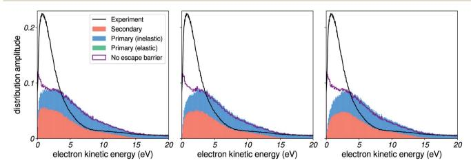
Fig. 9 Influence of the escape barrier. Comparison of simulated spectra to experimental results, for a photon energy corresponding to harmonic 37 of  $\approx$  800 nm ( $\approx$  57.6 eV), for several surface escape barriers. Left: 0.2 eV barrier. Middle: 0.5 eV barrier. Right: 0.8 eV barrier.
