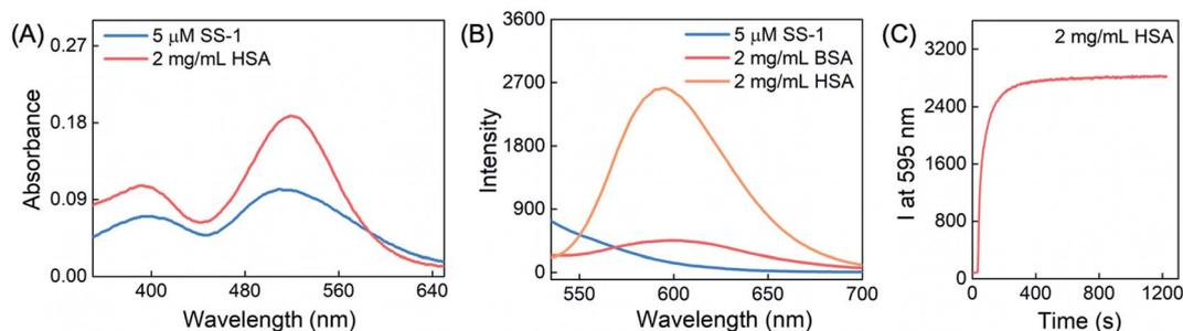
Fig. 1 Optical responses of **SS-1** toward HSA. (A) UV-vis absorption changes upon addition of 2 mg mL<sup>-1</sup> HSA into a 5 μM **SS-1**-containing PBS system. (B) The corresponding changes in the fluorescence spectra. (C) Time-dependent fluorescence intensity change in the reaction system at 595 nm.  $\lambda_{\text{ex}} = 505$  nm;  $\lambda_{\text{em}} = 525$ –700 nm; slit 5/5 nm; 700 V.
