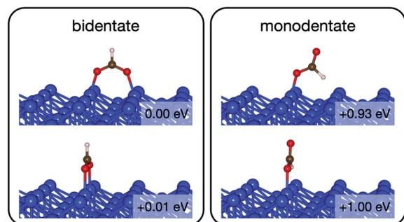
Fig. 8 The intermediate configurations of formate on Cu(110).
