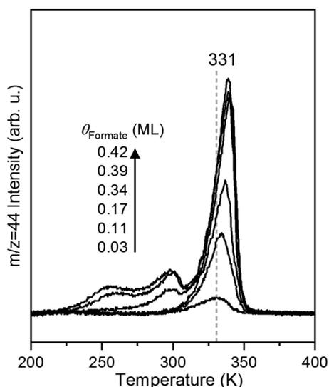
Fig. 3 The kinetics of CO<sub>2</sub> formation from formate decomposition depends on the initial coverage of oxygen on the Au(110) surface based on shifts in the peak temperature and development of multiple peaks. The formate coverages are 0.03, 0.11, 0.17, 0.34, 0.39 and 0.42 ML. Formic acid was dosed onto the oxygen-covered surface at 200 K followed by a linear heating at 1 K s<sup>-1</sup>.
