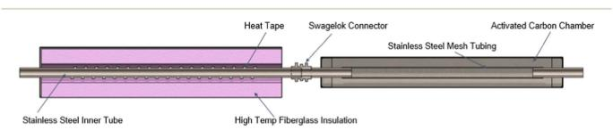
Fig. 2 Cross-sectional view of the thermodenuder used in the study, highlighting its different components. The temperature of the heating section was monitored *via* a K-type thermocouple placed at the mid-section surface of the sampling tube, providing feedback to an external temperature controller unit. The aerosol flow direction is from the left towards the denuder section to the right.
