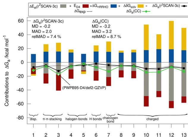
Fig. 5 Contributions to the association free energy  $\Delta G_a$  for each complex of the HS13L-CI in kcal mol<sup>-1</sup>. The statistical measures MD, MAD, relMAD, and for comparison,  $\Delta G_a$  based on “DLPNO-CCSD(T1)/CBS” energies instead of r<sup>2</sup>SCAN-3c are also given. For complex **3**, no coupled cluster values could be obtained and PWPB95-D4/def2-QZVP values are shown instead.
