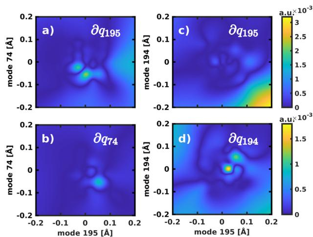
Fig. 6 Visualization of the NACs, projected into the 2D spaces spanned by normal modes 195/74 and 195/194, respectively. The notation  $\partial q_i$  refers to the projection of the NACs onto the respective normal mode to yield  $\langle \Psi_1 | \frac{\partial}{\partial q_i} | \Psi_2 \rangle$ .
