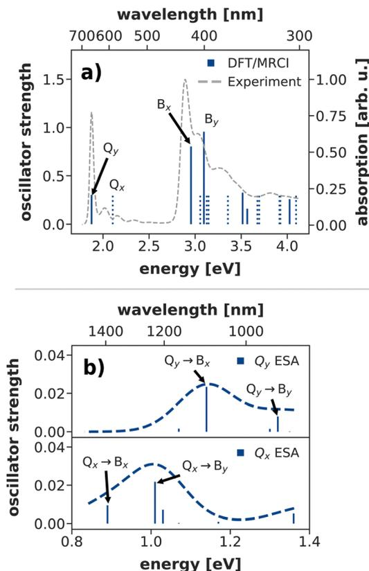
Fig. 3 (a) Calculated steady state absorption spectrum of a chlorophyll model system at the DFT/MRCI level of theory, compared to an experimental spectrum of chlorophyll *a* in diethyl ether.<sup>82,83</sup> The depicted absorption lines are red-shifted by 0.11 eV to the position of the experimental  $Q_y$  band. (b) Excited state absorption spectra from the Q-bands at the DFT/MRCI level of theory (unshifted).
