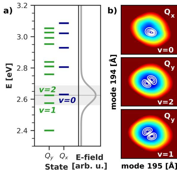
Fig. 10 (a) Vibrational energy levels of the electronic  $Q_y$  and  $Q_x$  states in a 2D space spanned by normal modes 195/194. The highlighted area illustrates the spectral width (FWHM) of the simulated laser pulse. Energies are given relative to the energy of the electronic ground state. (b) Visualization of the relevant vibrational eigenfunctions in the  $Q_x$  and  $Q_y$  potentials. Axis ranges and color scheme are identical to those in Fig. 9.
