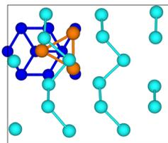
Fig. 6 Sketch of the commensuration of tellurene in the Te(10 $\bar{1}0$ ) geometry with the Si(111)-( $\sqrt{3} \times \sqrt{3}$ )R30°-Sb surface. The rectangular surface unit cell has edges  $a = 13.244$  Å and  $b = 11.470$  Å. For the silicon substrate only atoms within the surface unit cell in the first, second and fourth layers are shown.
