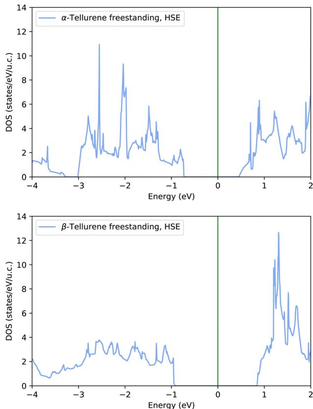
Fig. 8 Electronic density of states of the (top panel) 1T-MoS<sub>2</sub>-like ( $\alpha$ ) and (bottom panel) Te(10 $\bar{1}$ 0) ( $\beta$ ) phases of free-standing tellurene computed with the HSE06 functional and the tetrahedra method on  $64 \times 64$  ( $\alpha$  phase) or  $64 \times 48$  ( $\beta$  phase) meshes.
