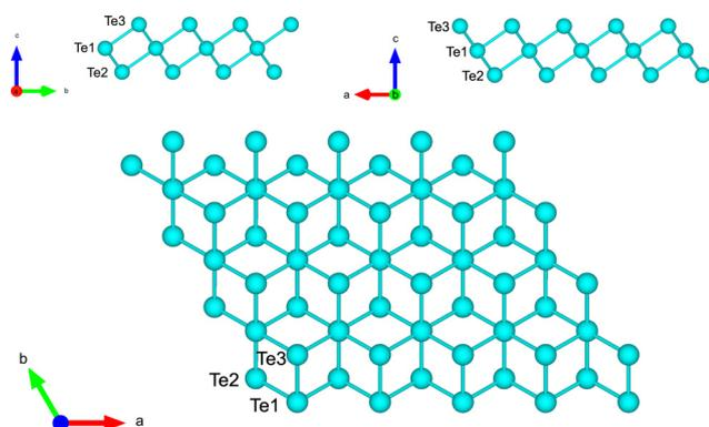
Fig. 2 Side and top views of the optimized structure of tellurene in the 1T-MoS<sub>2</sub>-like geometry. The three atoms per unit cell are labelled.
