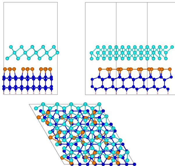
Fig. 5 The relaxed configuration of tellurene in a trilayer 1T-MoS<sub>2</sub>-like geometry adsorbed on the Si(111)-( $\sqrt{3} \times \sqrt{3}$ )R30°-Sb surface in a slab geometry. Side and top views are shown.
