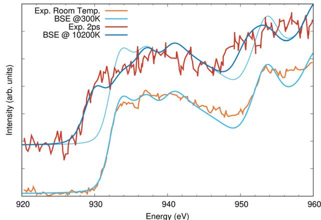
Fig. 5 Cu  $L_{2,3}$  edge X-ray absorption calculations compared to measured data taken from ref. 58. The lower spectra were taken and calculated at room temperature, while the upper spectra, offset vertically for clarity, are at elevated temperature (see text for details). The 300 K calculation is shown a second time with the high-temperature spectra to highlight the shifts in spectral weight with temperature.
