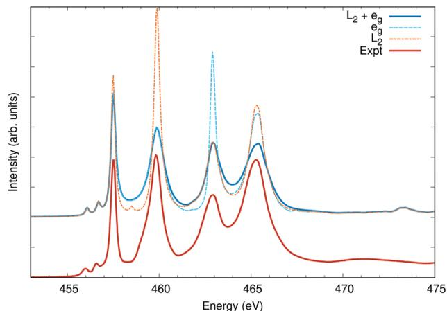
Fig. 8 The Ti  $L_{2,3}$  edge of  $\text{SrTiO}_3$  calculated using three different broadening methods compared to measured data taken from ref. 70. All calculated spectra have a uniform broadening of 0.25 eV full-width at half maximum. Selectively, peaks associated with the  $L_2$  edge ( $2p_{1/2}$  holes) are broadened to 0.52 eV, and peaks associated with the 3d  $e_g$  states are broadened by an additional 0.5 eV.
