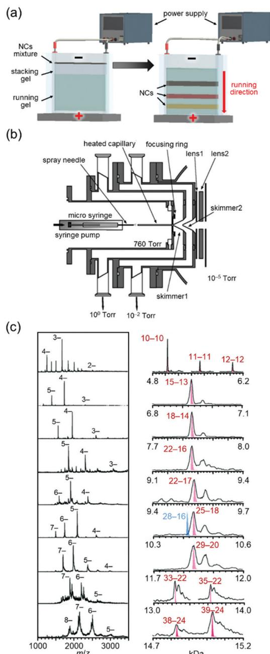
Fig. 3 (a) Schematic illustration of PAGE separation techniques.<sup>61</sup> (b) Details of the ESI source. (c) Negative-ion ESI mass spectrum of each fraction separated by PAGE.<sup>102</sup> In right figure, Au<sub>n</sub>(SG)<sub>m</sub> is described as n–m. Reproduced with permission from ref. 61 and 102. Copyright 2020 The Royal Society of Chemistry and 2005 American Chemical Society.
