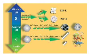
**Fig. 4** Schematic illustration of the growth mechanism and corresponding phase transitions of ZIFs and the derived oxides with different morphologies.
