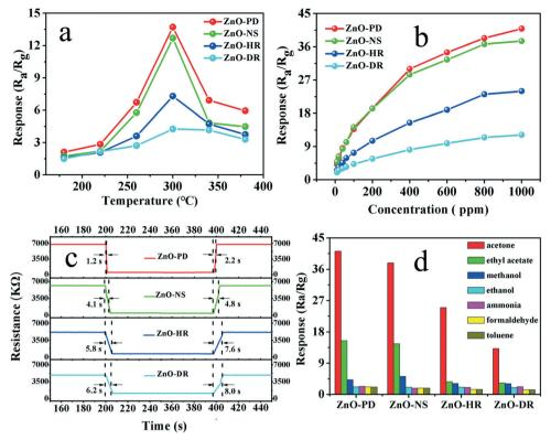
Fig. 7 (a) Sensitivities of the as-prepared samples toward 100 ppm acetone vapor at various operating temperatures. (b) Sensitivities of the asprepared samples to different concentrations of acetone vapor. (c) Response/recovery times of the sensors to 100 ppm acetone vapor. (d) Sensitivities of the as-prepared samples to various gases.
