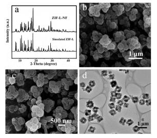
Fig. 1 XRD patterns (a), FESEM images (b and c), and TEM image (d) of ZIF-L-NF.
