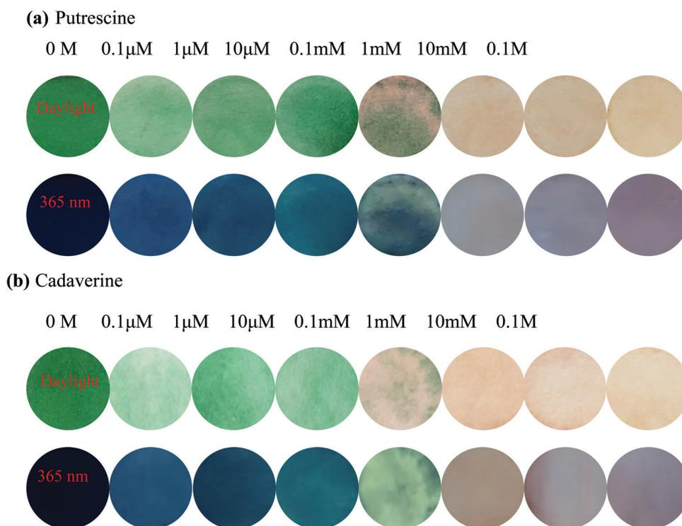
Fig. 6 The color and emission changes of the PPCy-1-loaded filter paper with colorimetric (top) and fluorescent (bottom) dual modes in the presence of (a) putrescine and (b) cadaverine solutions at  $25^\circ\text{C}$ .
