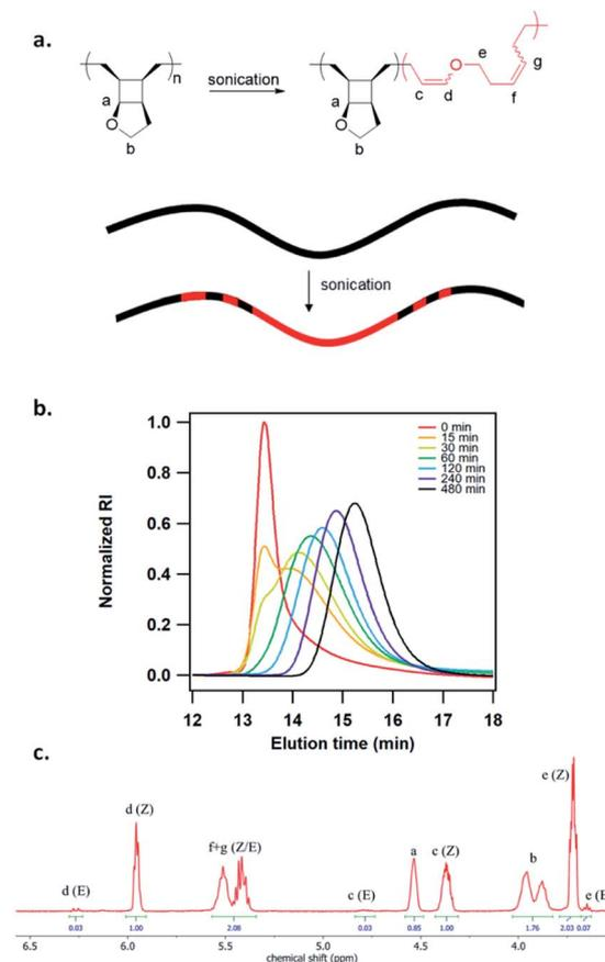
Fig. 2 (a) Mechanochemical activation of **P1-H** to generate poly(enol ether). (b) GPC traces of **P1-H** at different sonication times. (c) <sup>1</sup>H NMR spectrum of activated **P1-H** after 240 min of sonication.
