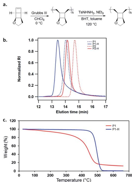
Fig. 1 (a) ROMP of monomer 1 and subsequent hydrogenation (the specified stereochemistry refers to that of the repeat unit, not suggesting the polymer tacticity). (b) GPC traces of poly(1) at different DPs and their hydrogenated polymers. (c) TGA traces of poly(1) and hydrogenated poly(1).
