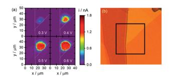
Fig. 6 Carrier confinement within more complex defect geometries. (a) CG-TC SECCM photocurrent images with the photoexcitation located near a triangular boundary within an n-WSe $_2$  nanosheet. (b) An optical transmission image of the same nanosheet, with the area interrogated  $\emph{via}$  SECCM indicated. Experimental parameters were identical to those employed in Fig. 2.
