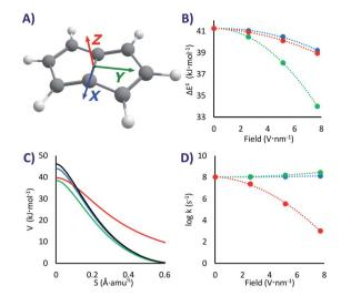
Fig. 2 (A) PL and the colour coded directing axes at which the EEF was applied. (B)  $\Delta E^{\ddagger}$  as a function of the field strength. (C) Potential energies at the M06-2x/6-311G(d) level vs. the reaction mass-scaled coordinates (only one side of the symmetrical PES is shown); in black the profile without EEF, blue, green and red are with 7.7 V nm $^{-1}$  fields in the X, Y, Z directions, respectively. (D) Tunnelling rate constants from the ground state vs. the field strength.
