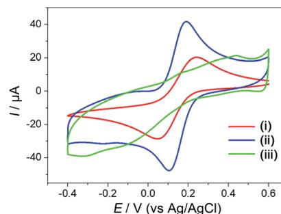
**Fig. 2** CVs obtained from different modified electrodes in 5 mM  $[\text{Fe}(\text{CN})_6]^{3-/4-}$  solution containing 0.1 M KCl and 0.1 M PBS at a scan rate of 100  $\text{mV s}^{-1}$ . (i) GCE, (ii) rGO/GCE, (iii) Hemin-doped-HKUST-1/rGO/GCE.
