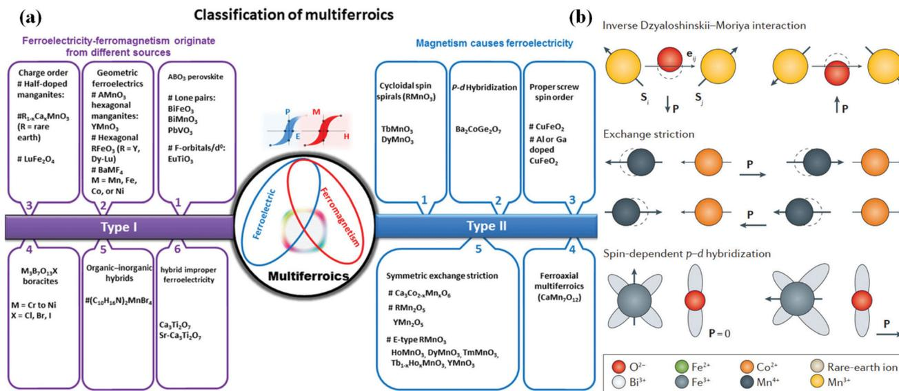
Fig. 5 Microscopic mechanisms of FE in type-II 2D multiferroics. (a) The classification of the multiferroic materials into two types with subclass groups. Reproduced with permission.<sup>60</sup> Copyright 2021, Springer Nature. (b) Three major microscopic mechanisms of FE in type-II multiferroic materials. Reproduced with permission.<sup>61</sup> Copyright 2014, IOP Publishing.
