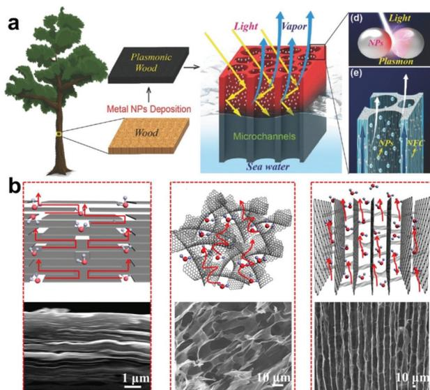
**Fig. 4** Water transport. (a) Schematic illustration of a plasmonic-wood-based evaporator. This figure has been reproduced from ref. 56 with permission from WILEY-VCH Verlag GmbH & Co. KGaA, Weinheim, copyright 2017. (b) Mechanism of the water transport channels of VA-GSM (right) and other rGO materials. This figure has been reproduced from ref. 18 with permission from American Chemical Society, copyright 2017.
