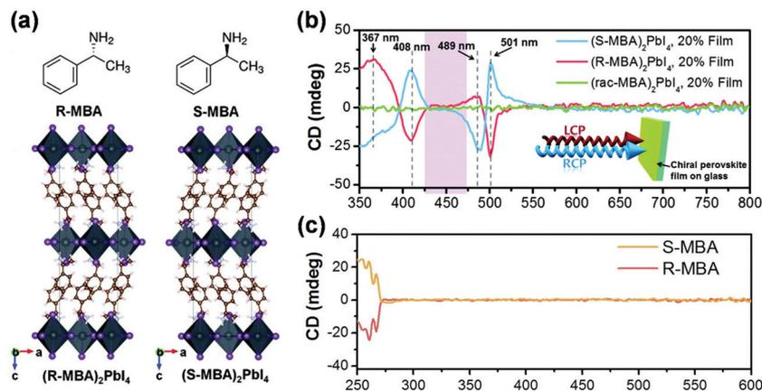
**Fig. 5** (a) Schematic illustration of the crystal structures of  $(R-/S\text{-MBA})_2\text{PbI}_4$  perovskites. (b) The CD spectra of  $(R-/S\text{-MBA})_2\text{PbI}_4$  and  $(\text{rac-MBA})_2\text{PbI}_4$  films. (c) The CD spectra of  $R-/S\text{-MBA}$ . This figure has been adapted/reproduced from ref. 18 with permission from Royal Society of Chemistry, Copyright 2017.
