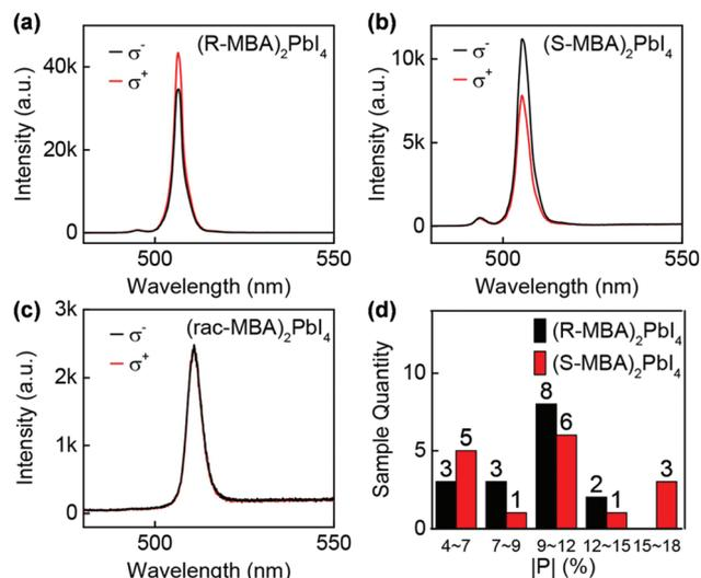
**Fig. 6** (a–c) The circularly polarized PL spectra of (R-MBA)<sub>2</sub>PbI<sub>4</sub>, (S-MBA)<sub>2</sub>PbI<sub>4</sub> and (rac-MBA)<sub>2</sub>PbI<sub>4</sub>, respectively under excitation of 473 nm laser at 77 K. (d) Statistical histogram of the degree of CPL emission (*P*) for (R-/S-MBA)<sub>2</sub>PbI<sub>4</sub>. This figure has been adapted/reproduced from ref. 70 with permission from American Chemical Society, Copyright 2019.
