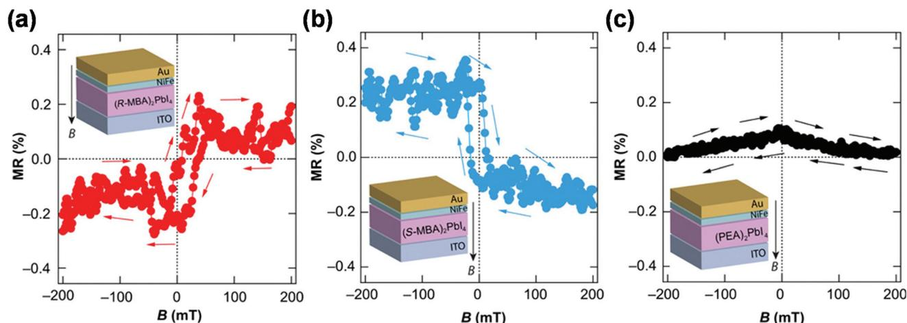
Fig. 12 The MR response towards the magnetic field in spin-valve devices based on the (a)  $(R\text{-MBA})_2\text{PbI}_4$ , (b)  $(S\text{-MBA})_2\text{PbI}_4$  and (c) achiral  $(\text{PEA})_2\text{PbI}_4$  perovskites, and the insets are the corresponding device structures. This figure has been adapted/reproduced from ref. 20 with permission from Science, Copyright 2019.
