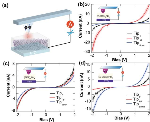
**Fig. 8** (a) Schematic illustration of mCP-AFM measurement setup, and (b-d) chirality-dependent out-of-plane charge transport based on 2D hybrid perovskite thin films of (*R*-MBA)<sub>2</sub>PbI<sub>4</sub>, (*S*-MBA)<sub>2</sub>PbI<sub>4</sub>, and achiral (PEA)<sub>2</sub>PbI<sub>4</sub>, respectively. This figure has been adapted/reproduced from ref. 20 with permission from Science, Copyright 2019.
