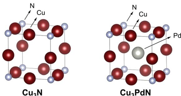
**Fig. 11** Crystal structure of  $\text{Cu}_3\text{N}$  and the doped  $\text{Cu}_3\text{PdN}$ . The copper is represented in dark red, the palladium in grey and the nitrogen atom in cyan. Structures plotted using VESTA.<sup>48</sup> Cif file obtained from ref. 111 and 112.
