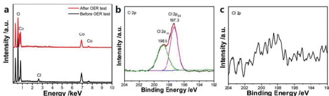
Fig. 12 (a) EDS analysis of Cl-doped  $\alpha$ -Co(OH)<sub>2</sub> catalyst in 1 M KOH solution. Cl 2p XPS spectra of the catalyst before OER test (b) and after the OER test (c).<sup>51</sup> Copyright © 2019, Royal Society of Chemistry.
