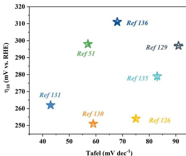
**Fig. 15** OER activity comparison graph showing the Tafel slope versus overpotential at a current density of 10 mA cm<sup>-2</sup> for different catalysts.
