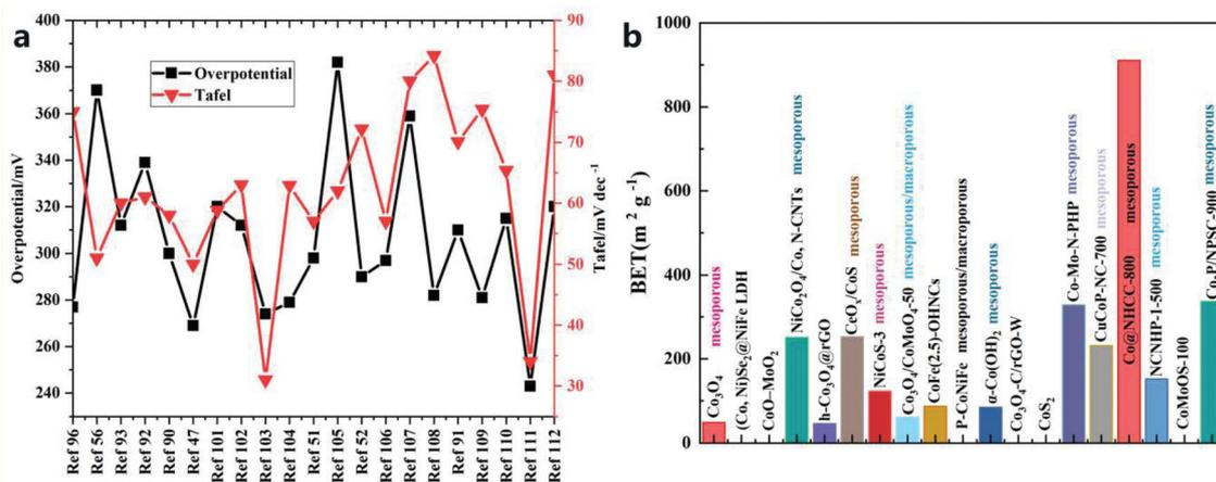
Fig. 9 Comparison of (a) Tafel slope and overpotential at a current density of 10 mA cm<sup>-2</sup> and (b) BET/BJH results for different catalysts.
