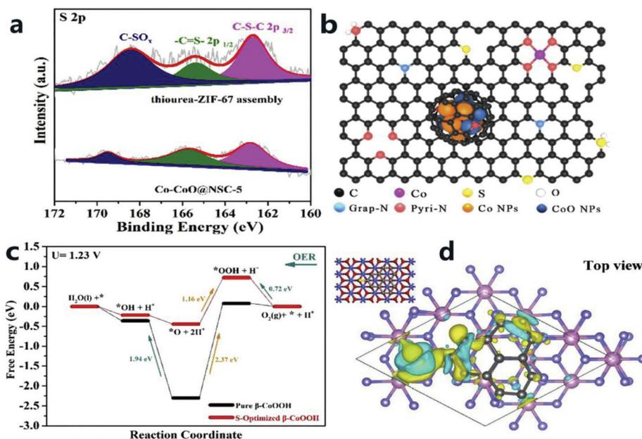
**Fig. 14** (a) S 2p XPS spectrum of thiourea-ZIF-67 component and Co-CoO@NSC-5. (b) Microscopic diagram of Co-CoO@NSC-5. (c) The calculated free-energy diagram of the OER on S-optimized  $\beta$ -CoOOH (001) ( $U = 1.23$  V). (d) The spin charge density distribution of  $\beta$ -CoOOH (001) (top view). Yellow indicates spin up and cyan indicates spin down.<sup>135</sup> Copyright © 2020 Elsevier B.V. All rights reserved.
