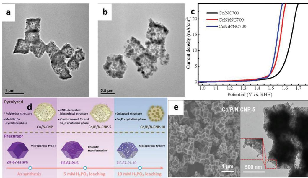
**Fig. 18** (a) TEM images of CoNi/NC700 and (b) CoNiP/NC700. (c) Polarization curves in KOH solution.<sup>155</sup> Copyright © 2018 Dalian Institute of Chemical Physics, the Chinese Academy of Sciences. Published by Elsevier B.V. All rights reserved. (d) Schematic illustration of a pre-leaching strategy for the preparation of Co/P/N–CNP catalysts. (e) SEM and TEM images of Co/P/N–CNP-5.<sup>136</sup> Copyright © 2020 Elsevier Ltd. All rights reserved.
