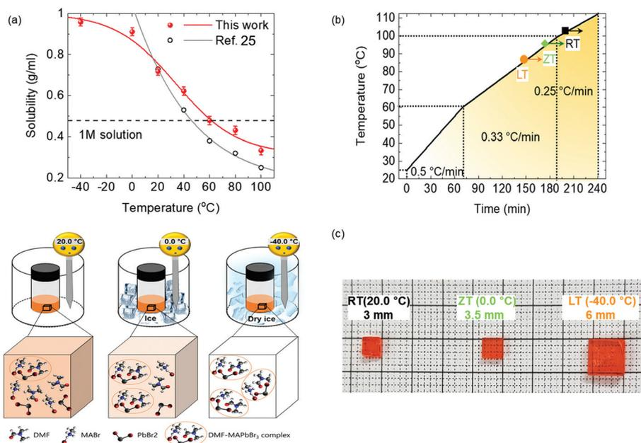
**Fig. 1** (a) Temperature-dependent solubility of MAPbBr<sub>3</sub> in DMF compared to ref. 21 and schematic diagram of dissolution temperature control, (b) heating rate of crystallization for high speed process, (c) MAPbBr<sub>3</sub> single crystal size at different dissolution temperatures.
