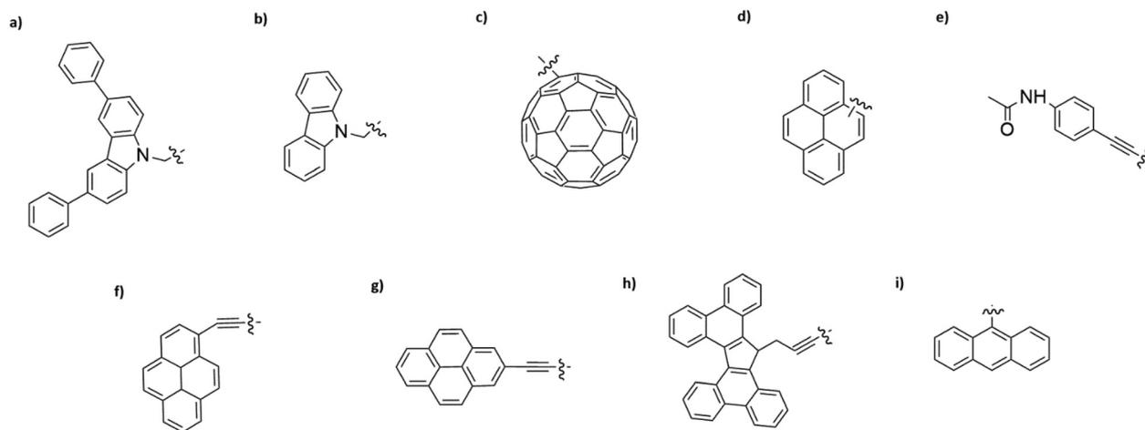
**Fig. 1** Examples of non-covalent anchoring groups used in graphene-based devices. (a) Biphenyl *N*-carbazole, (b) Carbazole, (c) Fullerene, (d) Pyrene, (e) Amine, (f) Pyrene-1, (g) Pyrene-2, (h) Tetrabenzofluorene, (i) Anthracene.
