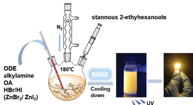
Scheme 1 Schematic diagram of the synthesis of the 2D (\text{RNH}_3)_2\text{SnX}_4 perovskites by a hot-injection method.
