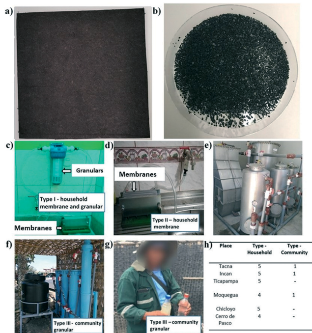
Fig. 2 (a) Photograph of the filtration membrane. (b) Photograph of the granular media. (c) Type I – household filtration unit (membrane and granular media). (d) Type II – household filtration unit (only the membrane). (e) Type III – community filtration unit in Torata. (f) Type III – community filtration unit (only granular) in Inclan. (g) Water samples collected from the Inclan area with high turbidity (sample in the left side: before filtration; sample in the right side: after filtration) and (h) the number of the household and community installations in the selected areas.
