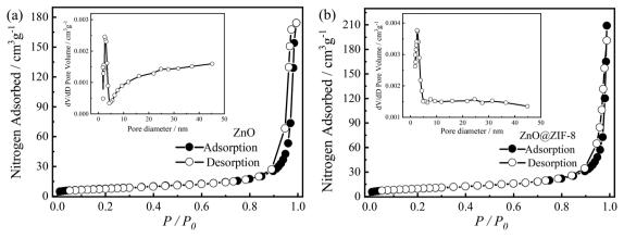
Fig. 4 Nitrogen adsorption-desorption isotherms of (a) ZnO and (b) ZnO@ZIF-8 core-shell nanorods. The insets show the corresponding pore size distributions.
