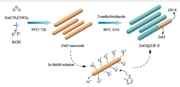
Fig. 1 Growth process of ZnO@ZIF-8 core-shell nanorods.
