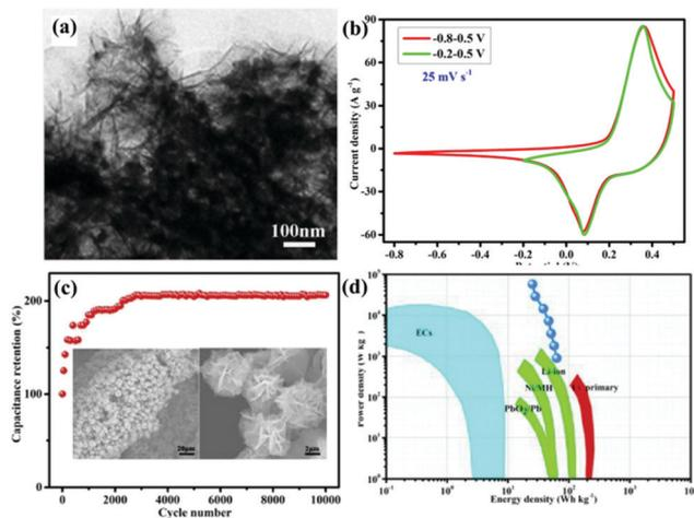
Fig. 9 (a) TEM images of LSM15@NC scratched down from the Ni foam. (b) Comparative CV curves at a scan rate of  $25 \text{ mV s}^{-1}$  within different potential windows of  $-0.8$  to  $0.5 \text{ V}$  and  $-0.2$  to  $0.5 \text{ V}$ . (c) Cycling performance (the insets show the morphology of LSM15@NC after 10 000 cycles). (d) Ragone plot. Reproduced from ref. 113 with permission from Elsevier B.V., copyright 2018.
