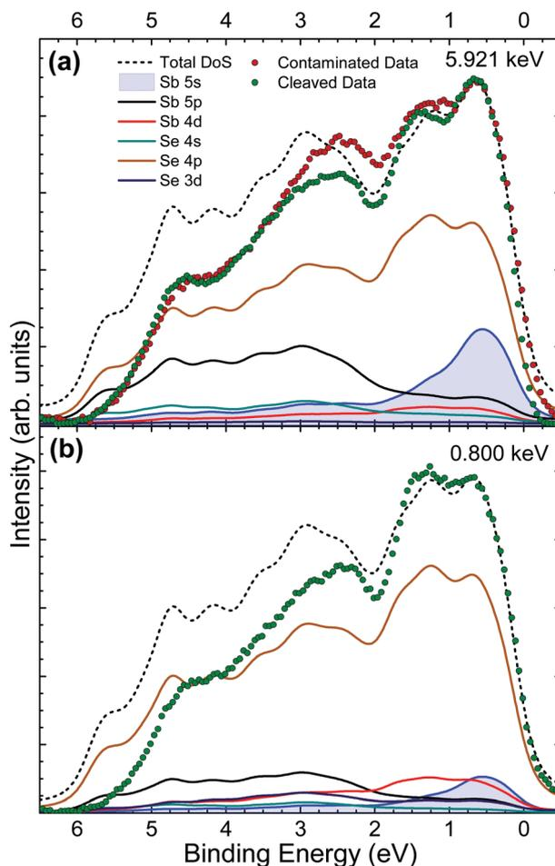
Fig. 5 VB XPS spectra from an  $\text{Sb}_2\text{Se}_3$  single crystal sample for (a) hard X-rays with a photon energy of 5.921 keV (HAXPES), before and after *in situ* crystal cleaving; and (b) soft X-rays with a 0.800 keV photon energy after *in situ* cleaving. Both are plotted with total and partial theoretical VB DoS calculations.
