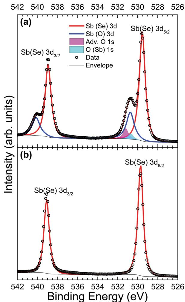
Fig. 3 Sb 3d HAXPES data from an Sb<sub>2</sub>Se<sub>3</sub> crystal (a) before and (b) after *in situ* cleaving.
