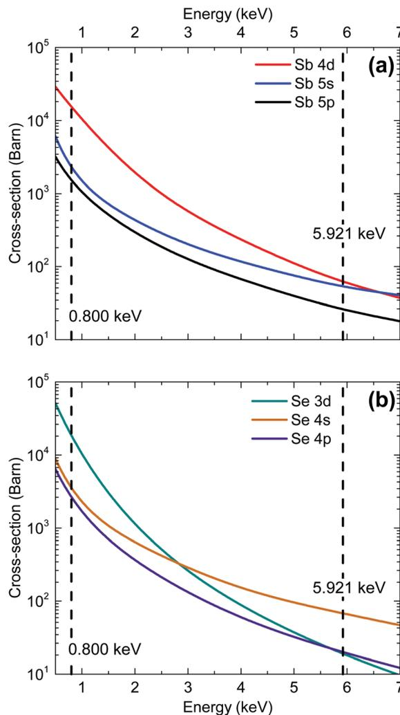
Fig. 2 Photoionization cross-section energy dependence for each valence orbital in (a) antimony and (b) selenium.<sup>25</sup>
