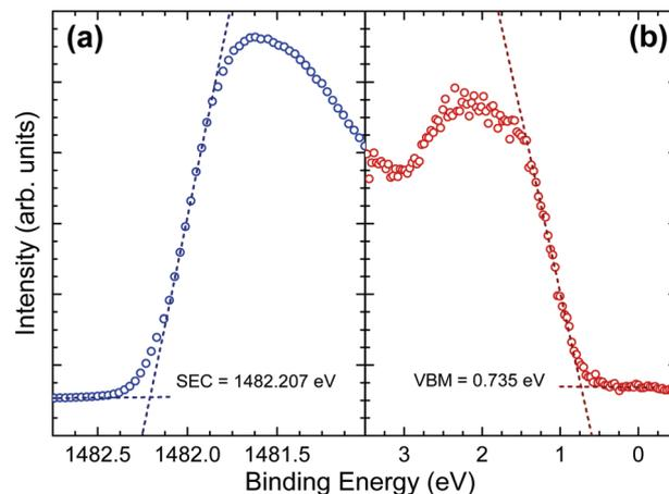
Fig. 6 (a) Secondary electron cut-off (blue) and (b) valence band maximum (red) of *in situ* cleaved  $\text{Sb}_2\text{Se}_3$  bulk crystals with straight line fits used to determine the binding energy of the cut-offs. The incident photon energy is 1486.6 eV.
