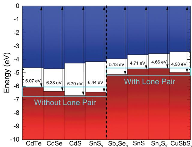
Fig. 7 Ionization potential for  $\text{Sb}_2\text{Se}_3$  from the photoemission results in Fig. 6, compared with literature values for other materials.<sup>23,24,49,50</sup> The zero of the energy scale corresponds to the vacuum level. The materials are labelled as without or with lone pair  $5s^2$  electrons.
