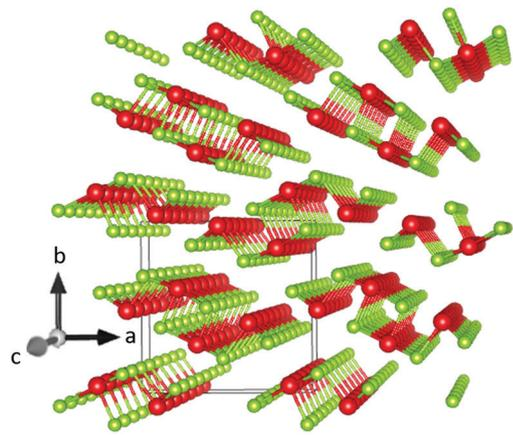
Fig. 1  $\text{Sb}_2\text{Se}_3$  crystal structure drawn in VESTA 3 (ref. 2) – antimony atoms are shown in red and selenium atoms in green. The solid line cuboid represents the unit cell. The axes labels correspond to the  $Pbnm$  setting of space group 62.
