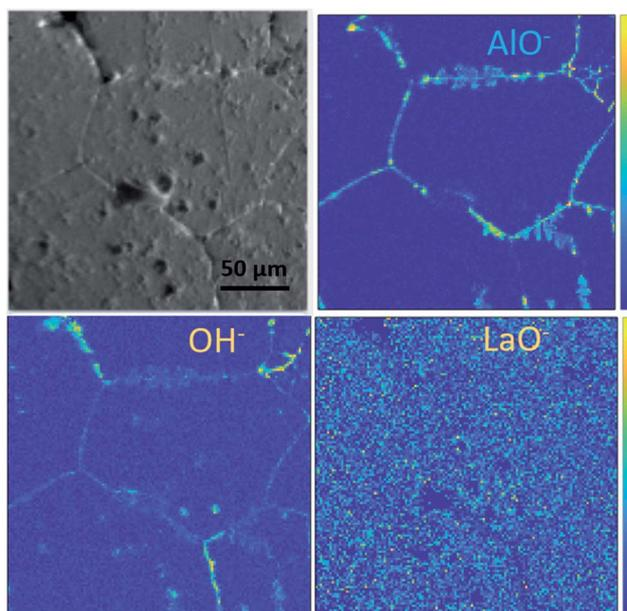
Fig. 7 ToF-SIMS negative secondary ion maps and optical image (greyscale) of an etched LLZO sample. The analysis was performed using 25 keV Bi<sup>+</sup> primary ions as the analytical beam and the sputtering was performed by 1 keV O<sub>2</sub><sup>+</sup> beam (burst mode).
