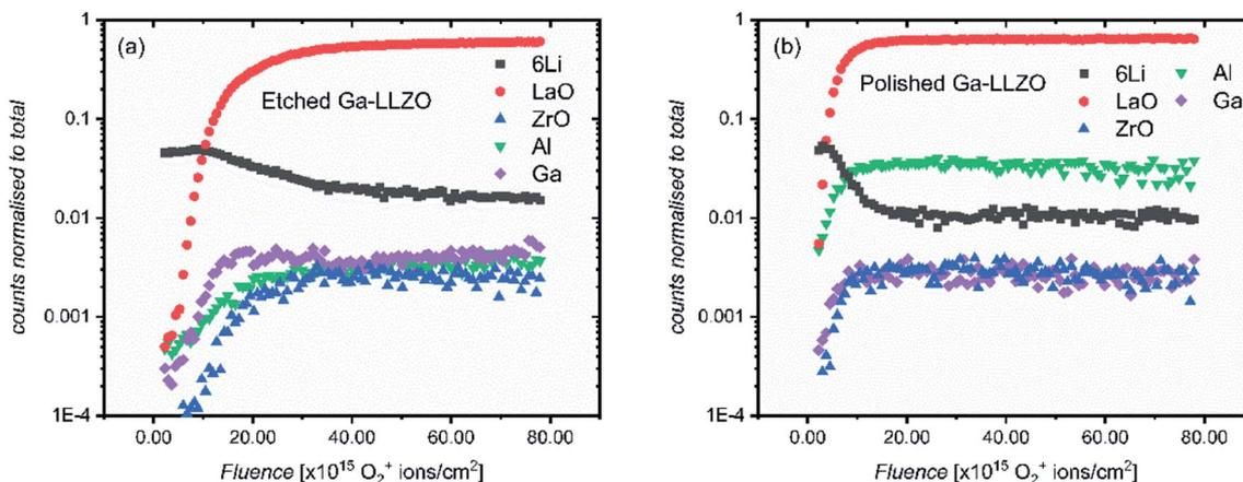
Fig. 4 ToF-SIMS depth profiles of etched (a) and polished (b) Ga-LLZO pellets, showing positive secondary ion species. The analysis was performed using 25 keV  $\text{Bi}^+$  primary ions as the analytical beam and the sputtering was performed by 1 keV 300 nA  $\text{O}_2^+$  beam (burst mode).
