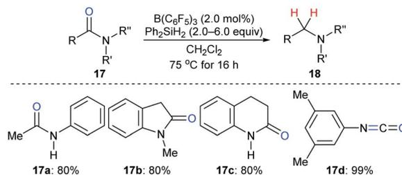
Scheme 15 Deoxygenation of amides and isocyanate catalysed by  $B(C_6F_5)_3$  with  $Ph_2SiH_2$  as the reductant.
