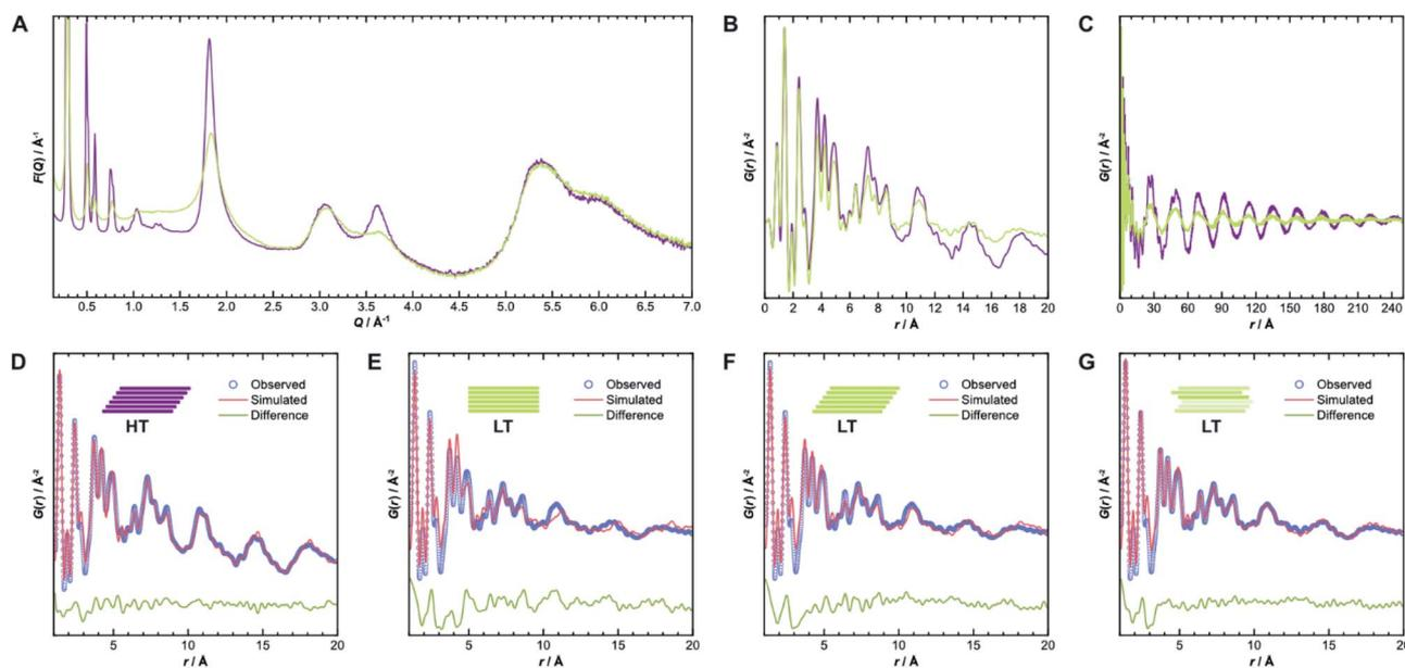
Fig. 5 (A) Comparison of reduced total scattering structure functions  $F(Q)$  for HT (purple) and LT (green) collected using synchrotron radiation. (B) Pair distribution functions derived thereof up to 20 Å and (C) up to 250 Å. (D) Best obtained PDF fits over 1–20 Å from structure refinements of HT, assuming unidirectionally slipped stacking, and (E) of LT, assuming eclipsed, (F) unidirectionally slipped, or (G) randomly slipped stacking.
