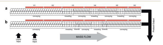
Fig. 2 (a) Schematic illustration of the standard screw configuration, and (b) the reverse screw configuration, used during the investigations and optimisation of the synthesis for CC3. The six heating zones down the length of the barrel are labelled (H1–H6).
