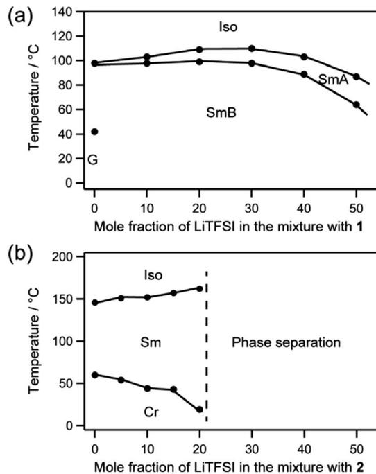
Fig. 5 Phase diagrams for mixtures of (a) **1** and (b) **2** with LiTFSI, determined with POM observation and DSC on cooling. SmB: smectic B; SmA: smectic A; Sm: unidentified smectic; Iso: isotropic; G: glass; Cr: crystal.
