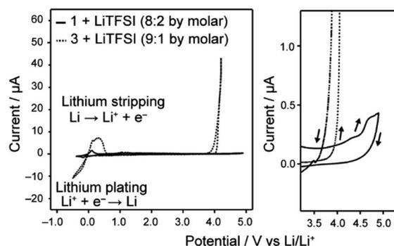
Fig. 3 Cyclic voltammograms of the LC electrolytes containing LiTFSI, recorded in the voltage region of –0.5–4.9 V vs. Li/Li<sup>+</sup> for **1**/LiTFSI and –0.5–4.2 V vs. Li/Li<sup>+</sup> for **3**/LiTFSI, respectively. Enlarged curves in the high voltage region are shown at the right part. Arrows in the right part indicate the sweep direction of cyclic voltammograms.
