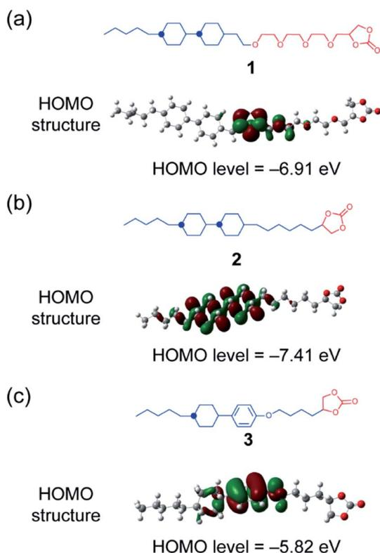
Fig. 2 (a and b) Molecular structures and HOMO levels of molecules **1** and **2** in the present study. (c) Compound **3**, which was a previously developed LC molecule for the application of electrolytes in Li-ion batteries,<sup>9</sup> is shown for reference.
