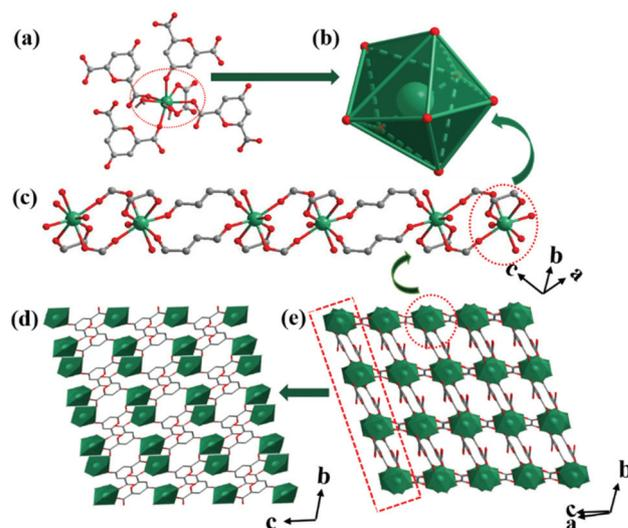
**Fig. 1** Coordination environment (a) and coordination geometry (b) of  $\text{Tb}^{3+}$  ion; (c) the connection mode of  $\text{TbO}_8$ ; (d) 2D layer of Tb-MOF along the  $a$  axis; (e) 3D framework of Tb-MOF. Atom codes: Tb (green), O (red), C (gray). Hydrogen atoms are removed for clarity.
