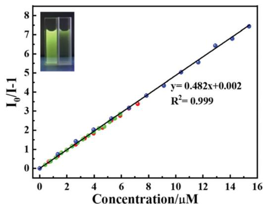
Fig. 4 Summary of S–V plots at 544 nm of Tb-MOF towards nitrite ions with different volumes, 3  $\mu\text{L}$  (green plots), 5  $\mu\text{L}$  (red plots), 10  $\mu\text{L}$  (blue plots). Inset is the picture of Tb-MOF suspension excited by 254 nm ultraviolet light before and after adding 20  $\mu\text{L}$  nitrite aqueous solution (4 mM).
