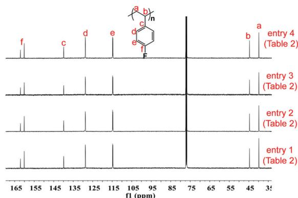
Fig. 1 <sup>13</sup>C NMR spectra of poly(*p*FSt) (125 MHz, CDCl<sub>3</sub>, 25 °C).
