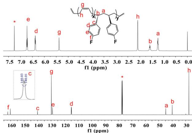
**Fig. 3** <sup>1</sup>H and <sup>13</sup>C NMR spectra of poly(*p*FSt-BD) (Table 1, entry 4) (500 MHz for <sup>1</sup>H NMR and 125 MHz for <sup>13</sup>C NMR, CDCl<sub>3</sub>, 25 °C).
