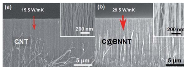
Fig. 13 Scanning electron microscopy (SEM) images of (a) VA-CNTs and (b) VA-MWCNTs coated in h-BN. The h-BN coating increased thermal conductivity of the aligned assembly from  $15.5\text{ W m}^{-1}\text{ K}^{-1}$  to  $29.5\text{ W m}^{-1}\text{ K}^{-1}$ . Reproduced with permission from ref. 22. Copyright 2017, American Chemical Society.
