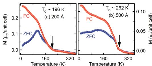
Fig. 2 Temperature dependence of the out-of-plane zero-field-cooled and field-cooled magnetization of the 200 and 500 Å thick  $\text{La}_{0.7}\text{Sr}_{0.3}\text{MnO}_3$  films grown on (001) oriented  $\text{LaAlO}_3$  in the presence of a 0.01 T field.
