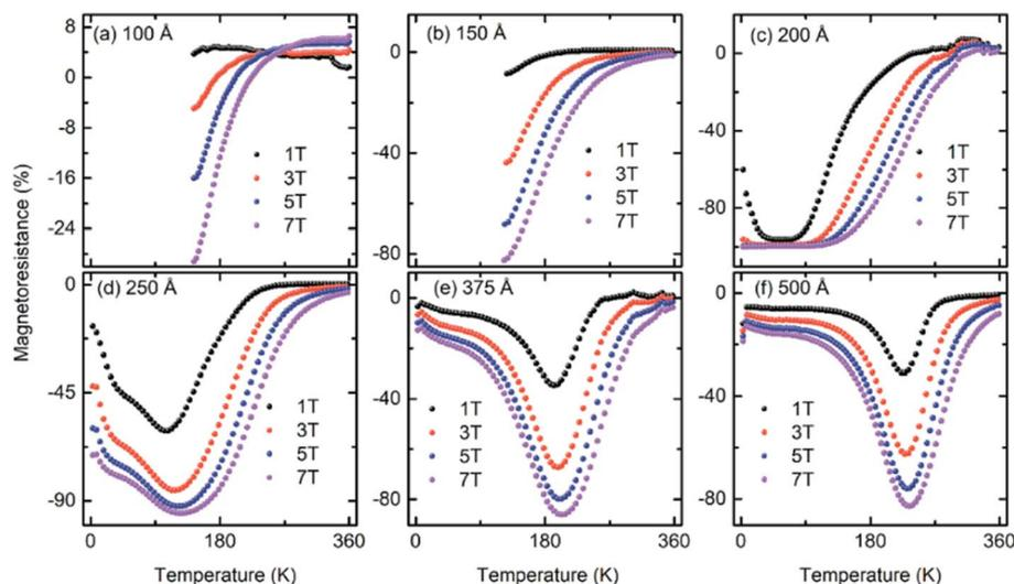
**Fig. 6** Temperature-dependent magnetoresistance of the (a) 100 Å, (b) 150 Å, (c) 200 Å, (d) 250 Å, (e) 375 Å, and (f) 500 Å thick  $\text{La}_{0.7}\text{Sr}_{0.3}\text{MnO}_3$  films grown on (001) oriented  $\text{LaAlO}_3$  measured in the presence of 1, 3, 5, and 7 T magnetic fields.
