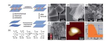
Fig. 4 (a) Illustration of the synthetic process of 2D MOFs by using the electrochemical/chemical exfoliation method and (b) a possible oxidative transformation route from H<sub>4</sub>dhbdc to a species with m/z 168. SEM images of (c) 3D-Co, (d) 2D-Co, and (e) 2D-Co-NS. (f) TEM image of 2D-Co-NS (inset: Tyndall effect of a colloidal solution). (g) AFM image and (h) the corresponding height profile of 2D-Co-NS. Reproduced with permission.77 Copyright@2018 WILEY-VCH Verlag GmbH & Co. KGaA.
