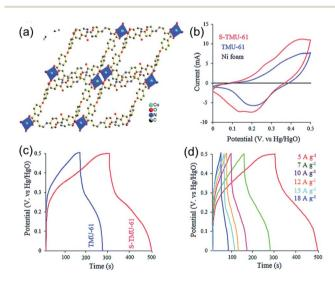
Fig. 14 (a) Topological diagram of TMU-61. (b) CV curves of TMU-61, S-TMU-61, and Ni foam at a scan rate of 25 mV s $^{-1}$ , (c) GCD curves of TMU-61 and S-TMU-61 electrode materials at a current density of 5 A g $^{-1}$  and (d) GCD curves of S-TMU-61 at different current densities. Reproduced with permission. Copyright 2019 The Royal Society of Chemistry.
