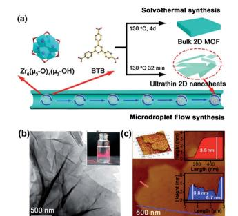
Fig. 12 (a) Schematic illustrations of the overall process developed to produce 2D MF-ZrBTB and ST-ZrBTB via microdroplet flow reaction and conventional solvothermal methods. (b) TEM image of MF-ZrBTB. The inset shows the Tyndall light scattering effect of MF-ZrBTB colloidal suspension. (c) AFM image and corresponding height profiles of MF-ZrBTB nanosheets along the red and blue lines. Reproduced with permission. 104 Copyright © 2018 American Chemical Society.
