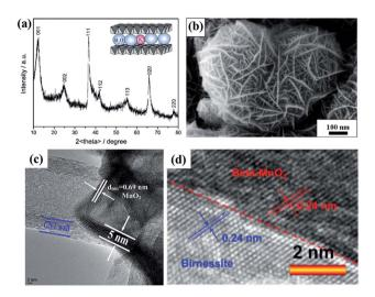
Fig. 2 (a) Typical XRD pattern of birnessite. 65 (b) SEM image of typical birnessite.<sup>67</sup> (c) and (d) HRTEM images of typical birnessite.<sup>49,68</sup>
